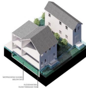
Install Flood Vents
